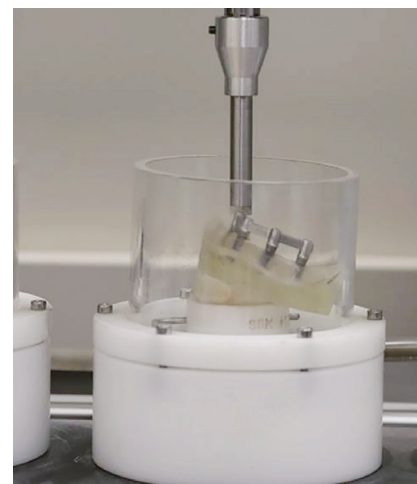
Fig. 4. Positioning of the model in the cyclic loading chewing simulator (CS-4) with 30 degrees angle.
