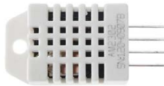
Fig. 5. Humidity and Temperature Sensor DHT22
