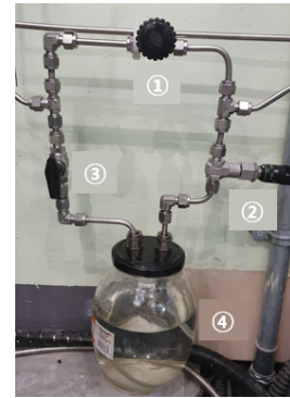
[Figure 3] Humidifier used in this study (① needle valve, ② micro needle valve, ③ ball valve, ④ bottle with water)
