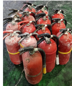
[Figure 1] Experimental materials according to the Expiration date of Powder Extinguisher
