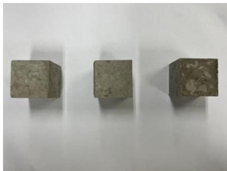
(a) Dry curing
