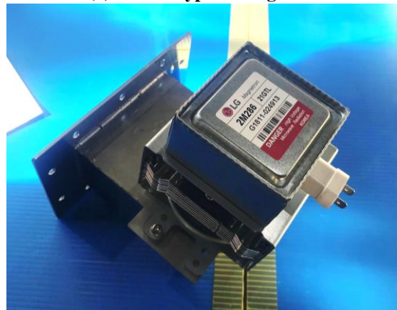
(b) waveguide assembled with magnetron
