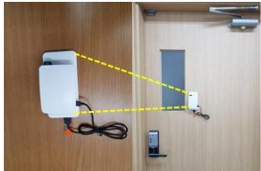
Fig. 4. Implemented WiFi extender and installation
