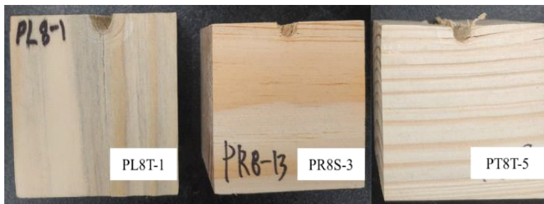
Fig. 6. Failure mode of tested specimens. PL: specimen of the cross section, PR: specimen of the radial section, PT: specimen of the tangential sections.
