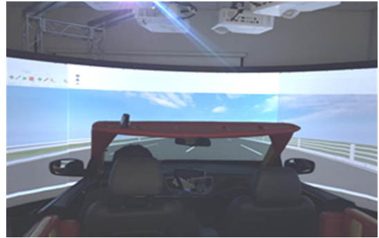
Fig. 3 Fixed-based driving simulator
