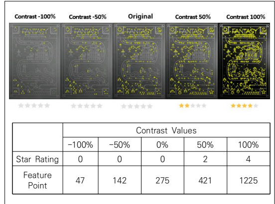
Fig. 6. Figure of the change in recognition rate according to the contrast values of the marker images
