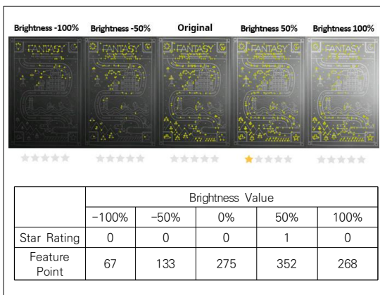
Fig. 10. Figure of the change in recognition rate according to the brightness values of the marker images
