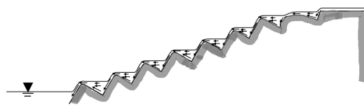
Fig. 8. Flow structure in baffles and pools
