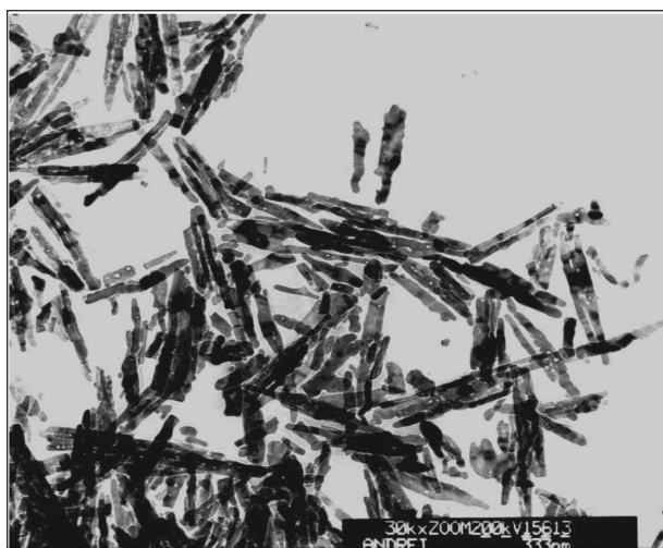
Fig. 2. Cryo-TEM image of Co- \gamma -Fe 2 O 3 particle in the magnetic dispersion.
