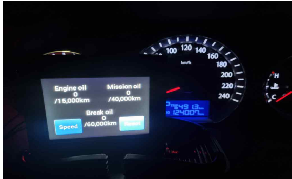
Fig. 11 Comparison of car maintenance support system and instrument cluster
