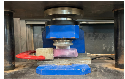
Figure 3. Measurement of Ice Attachment Loads
