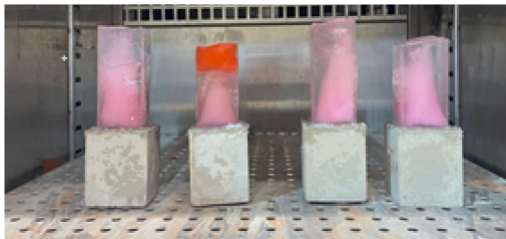
Figure 2. Fabrication of Ice Adhesion Performance Test Specimen
