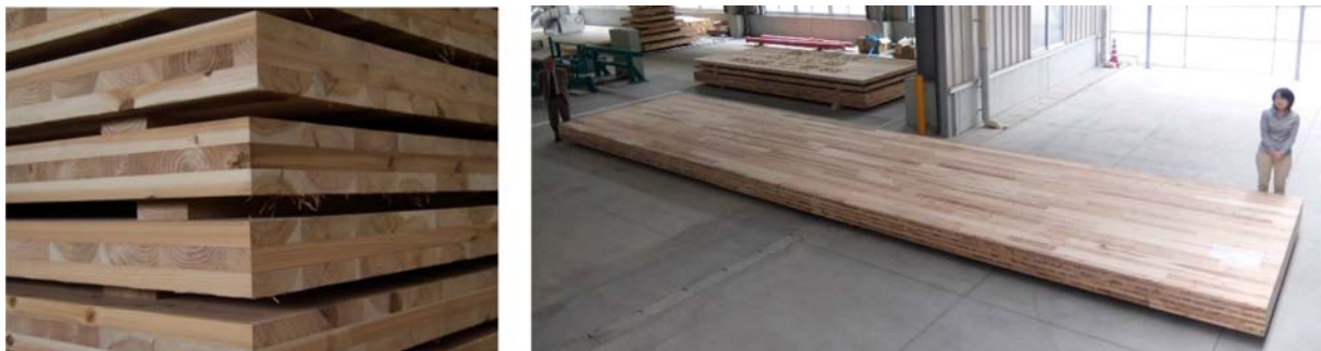
Figure 3. Cross laminated timber (CLT) and the maximum size of CLT panel fabricated in Japan. ( 3 \text{ m} \times 12 \text{ m} )
