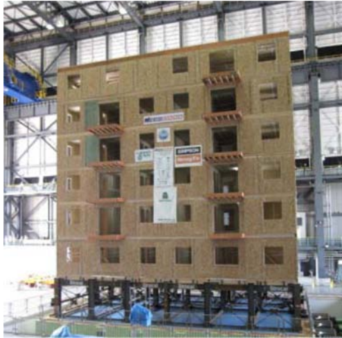
Figure 5. Full-scale shaking table test on 7-story wooden building at E-defense in 2009. (First story is steel structure)
