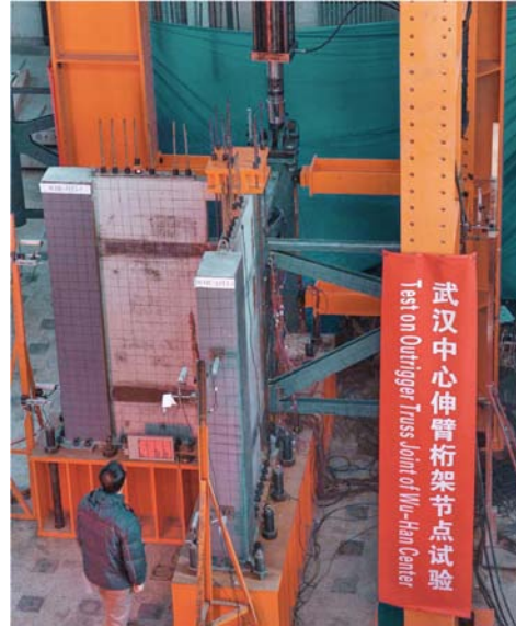
Figure 13. Outrigger-shear wall joint test.
