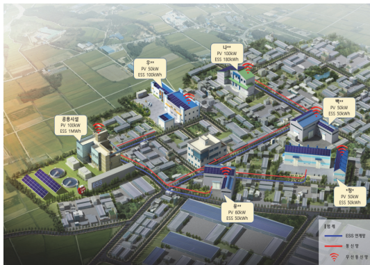
Fig. 2 Configuration of industrial complex microgrid
