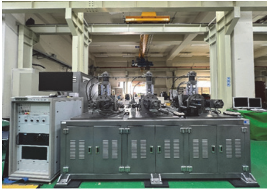
Fig. 3 Test mechanism of bearing durability
