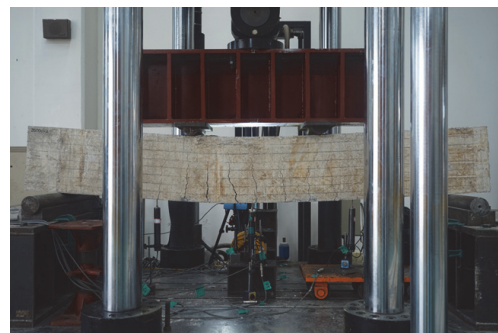
Fig. 4 Crack at the end of experiment
