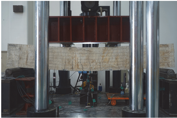
Fig. 4 Crack at the end of experiment
