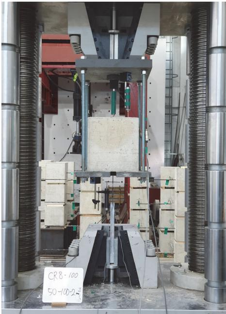
Fig. 4 Direct pull-out test setup of grid typed CFRP
