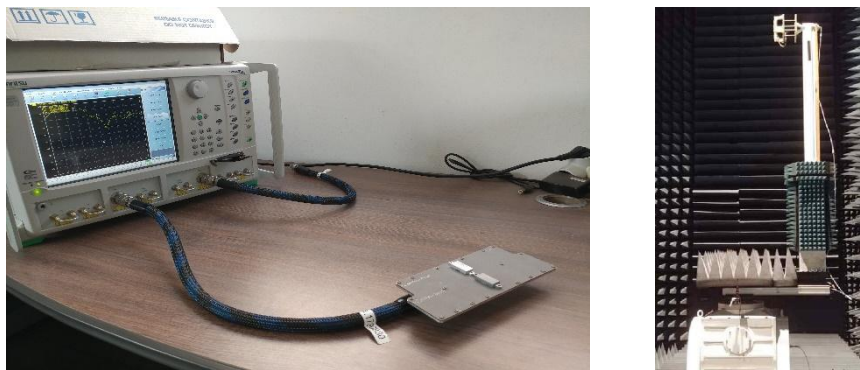
Figure 4. Measurement of Antenna Return loss & Gain
