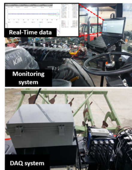
Fig. 2 Schematic diagram of engine load measurement system
