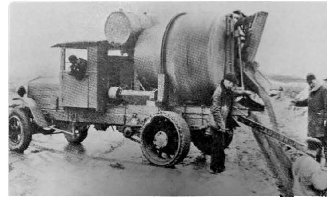
Designed and constructed by Chain Belt Company in 1930, this truck mixer had a capacity of three cubic yards. The design was superior to the Tumblebug in that it had a higher level discharge chute and didn't require a hydraulic hoist.
