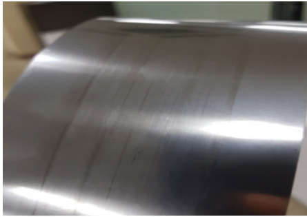
Fig. 11. The steel band worn by normal type mover.
