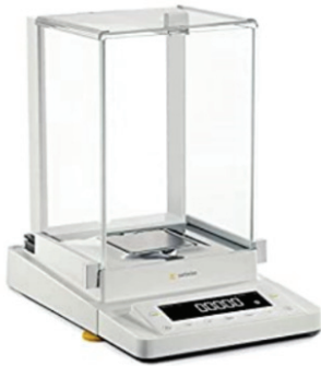
Fig. 7. The measuring equipment used in weighting steel Band.
