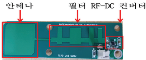
Fig. 1. Microwave wireless power receiver configuration..
