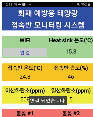
Fig. 7. WiFi monitoring system.
