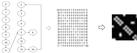
Fig. 4. CFG to image using adjacency matrices.
