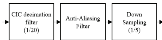
Fig. 7. Block diagram of the second proposed decimation filter.
