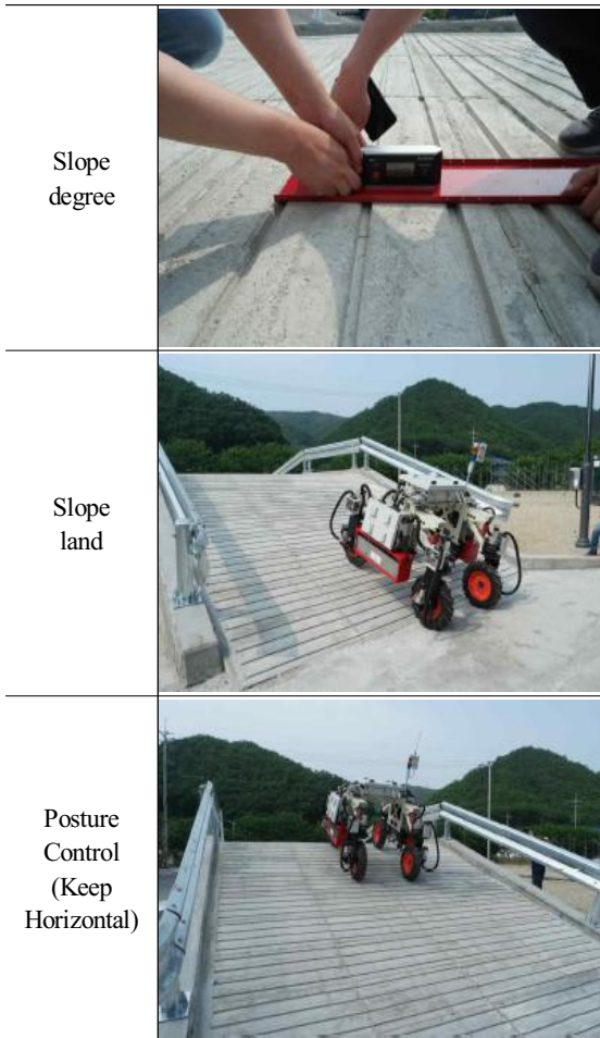
Fig. 8 Slope test of platform
