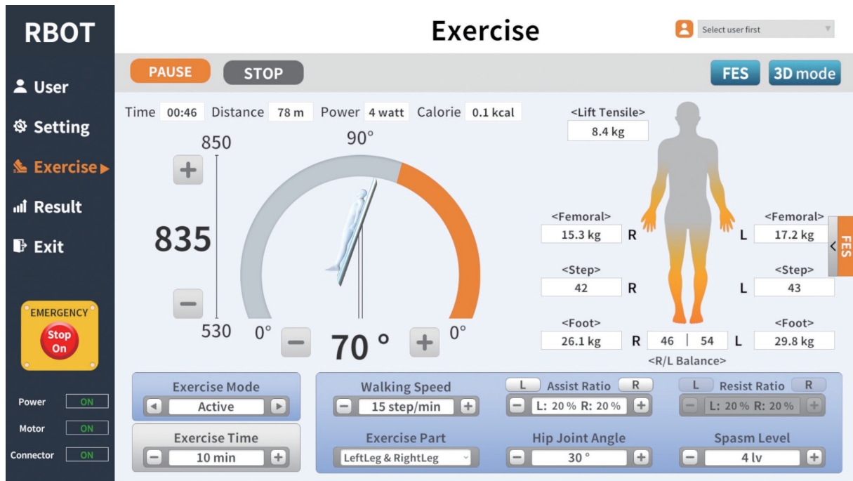
Figure 2. Robot assisted monitor. Active mode provides an assist ratio.
