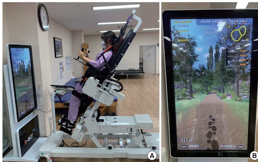
Figure 1. Robot intervention. (A) Side view during gait training using robot, (B) Provides visual feedback through footsteps.
