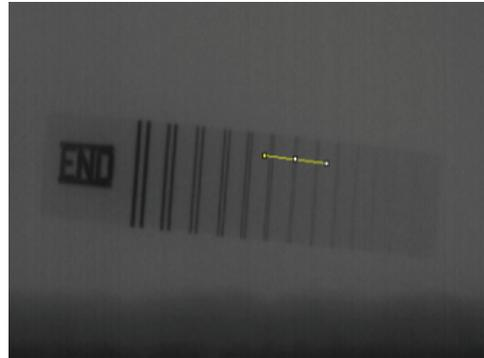
Fig 5. Profile area of Duplex Wire IQI D6, D7, D8.
