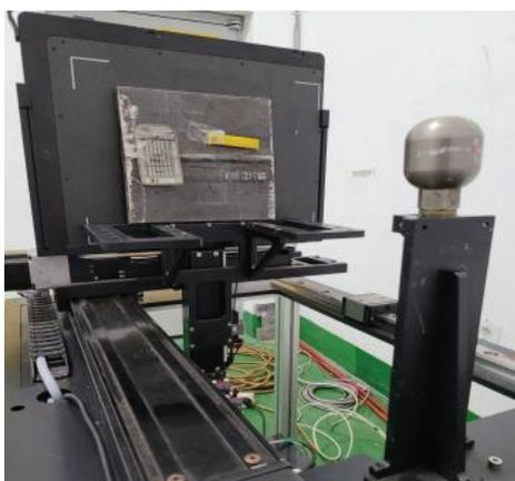
Fig. 2. Digital Radiography of Collimator, Weld Test Piece and Detector.
