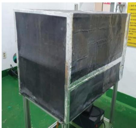
Fig. 3. Digital Radiography with Lead Shielding.
