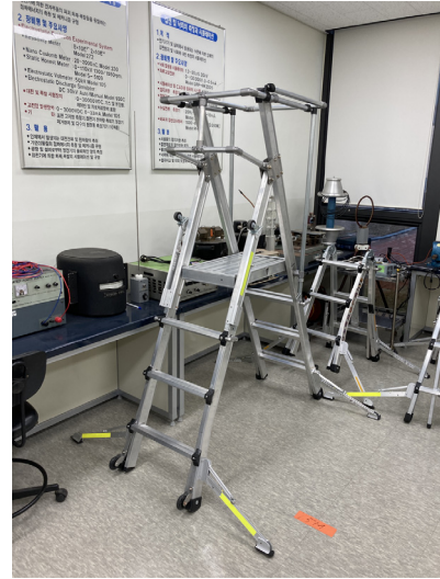
Fig. 3. Developed active platform ladder (Fabricated).
