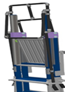
Fig. 5. Configuration of straightly foldable structure.
