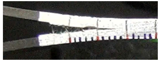
Fig. 9. Crack growth of DCB specimen
