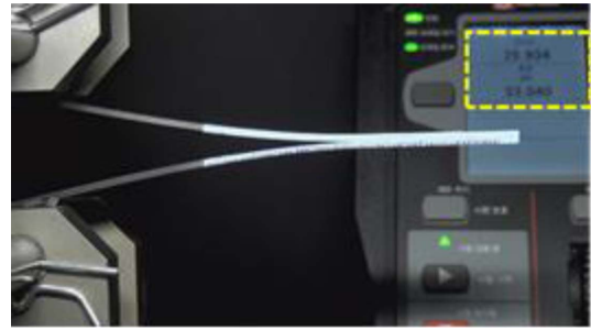
Fig. 6. Measurement of DCB test data using a high-resolution camera
