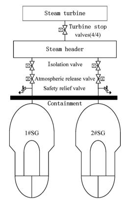
Fig. 5. Typical diagram of main steam lines with steam header.
