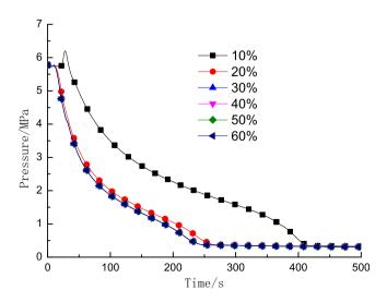
Fig. 12. Effects of the break scale on steam pressure of broken SG.
