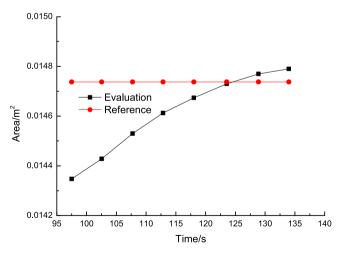
Fig. 9. Evaluation of break area for 2.5% scale MSLB.
