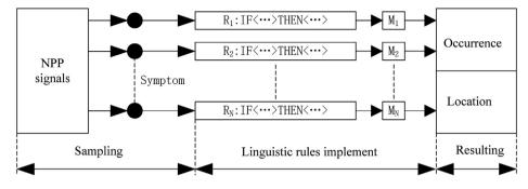
Fig. 3. Structure of the accident diagnosis logic.
