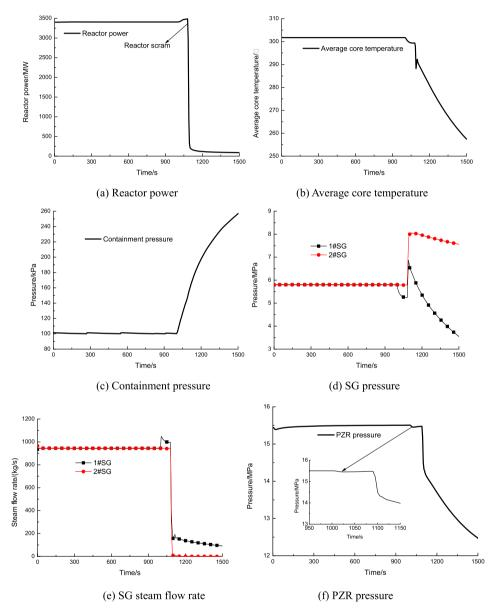
Fig. 2. Characteristics of the accident symptoms.
