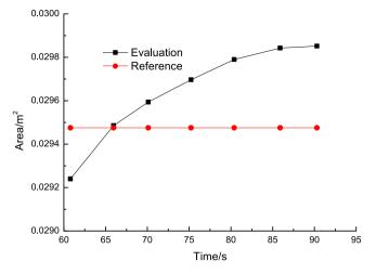
Fig. 10. Evaluation of break area for 5.0% scale MSLB.
