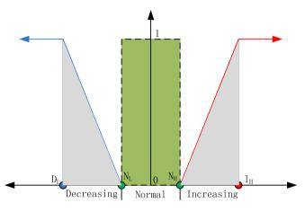
Fig. 4. Parameterized model for accident symptoms.
