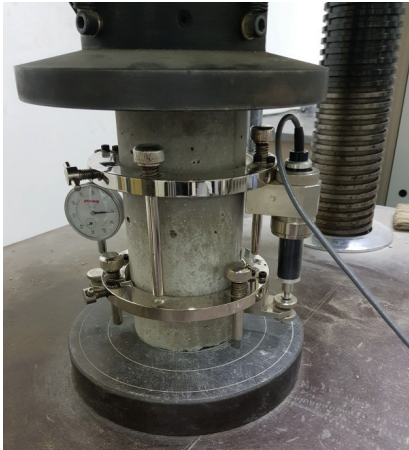
Fig. 1. Compressive displacement measurement
