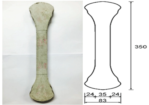
Fig. 4. Detail of specimen for direct tensile test
