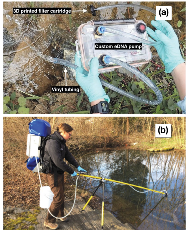
Fig. 7. Developed sampling pump for eDNA in freshwater. (a) Hand-held eDNA pump and associated 3D-printed filter cartridge and vinyl tubing (Edmunds et al. , 2019), (b) environmental DNA sampling using the ANDe™ system (Thomas et al. , 2018).
