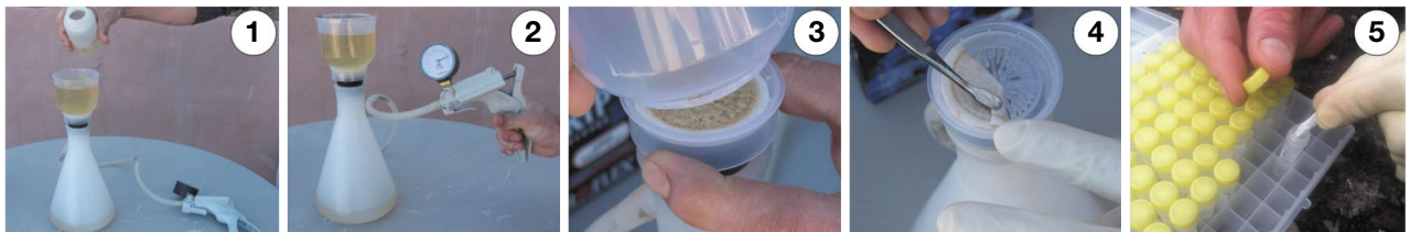
Fig. 4. Use of a hand pump for eDNA sampling. (1) Pour sample slowly into filter funnel, (2) Engage hand pump to begin filtration, (3) Remove funnel cup, (4) Fold filter, (5) Place filter in 2 mL o-ring tube of ethanol (Goldberg et al. , 2017).
