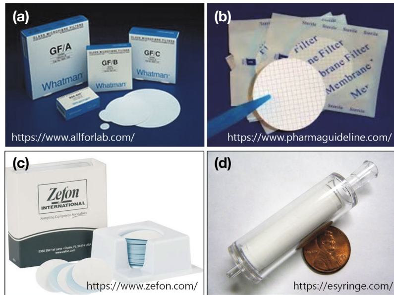
Fig. 2. Various type of filter paper and Sterivex filter. (a) Glass fiber filter paper, (b) Cellulose membrane filter paper, (c) Polycarbonate filter paper, (d) Sterivex filter set.
