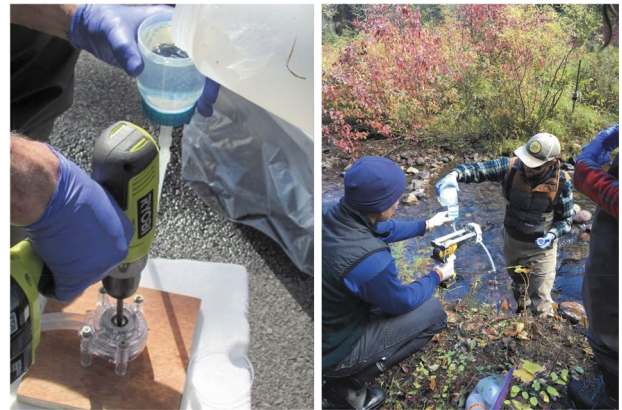
Fig. 6. eDNA filtration using a peristaltic pump support by power drill.
