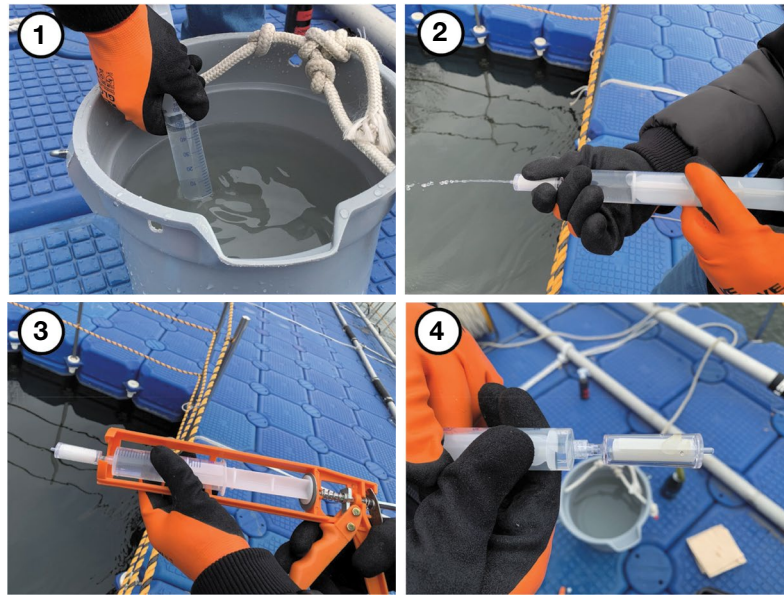
Fig. 3. Use of a Sterivex filter for sampling of eDNA in Water column. (1) Injection of field sampling to syringe, (2) Injection of water sample to Sterivex filter, (3) When you hard to push, using silicon injector, (4) Injection of preservation solution.
