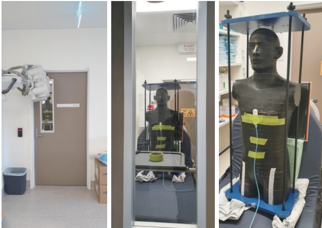
Fig. 1. Photographs showing (left to right) tube location outside room, phantom as viewed through window, phantom with dosimeter at sternum.
