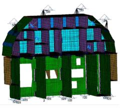
Fig. 9 Finite Element Model, Galley
