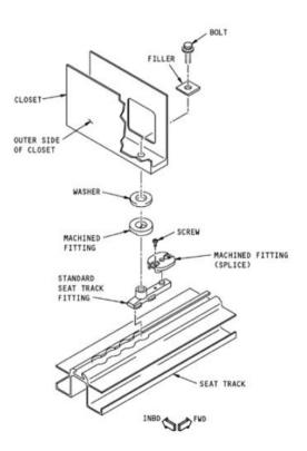
Fig. 7 Galley Structure Lower Attachment Design
