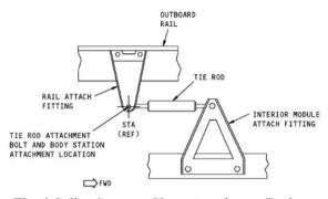
Fig. 6 Galley Structure Upper Attachment Design
