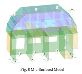
The design was modified such that the lower fitting part transfers all loads in the direction of the X, Y, and Z axes according to the movement of the structure, using the design concept applied as the tightening area boundary conditions, and one of the lower vertical panels, where a large displacement value is generated additionally and takes charge of the Y-directional load.
