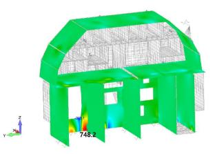
Fig. 16 Panel Flexure Bending Result
