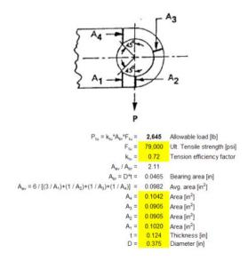
Fig. 13 Lug Allowable Calculation [9]
