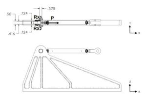
Fig. 12 Free Body Diagram, Upper Fitting
