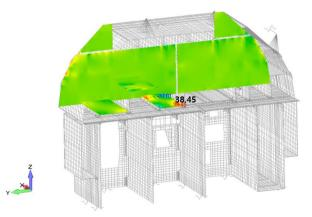
Fig. 17 Panel Core Shear Result
