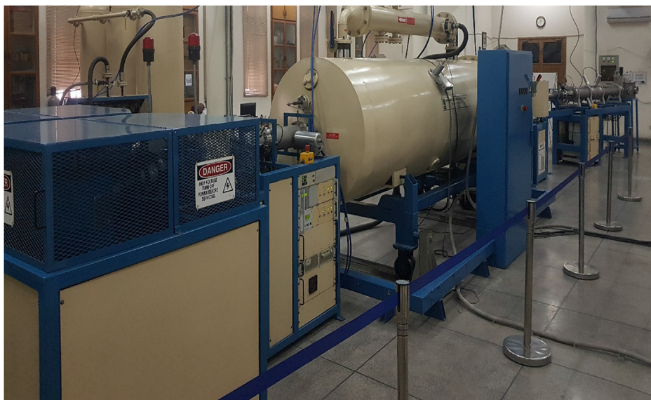
Fig. 1. Image of Pelletron Accelerator used for Irradiation.
