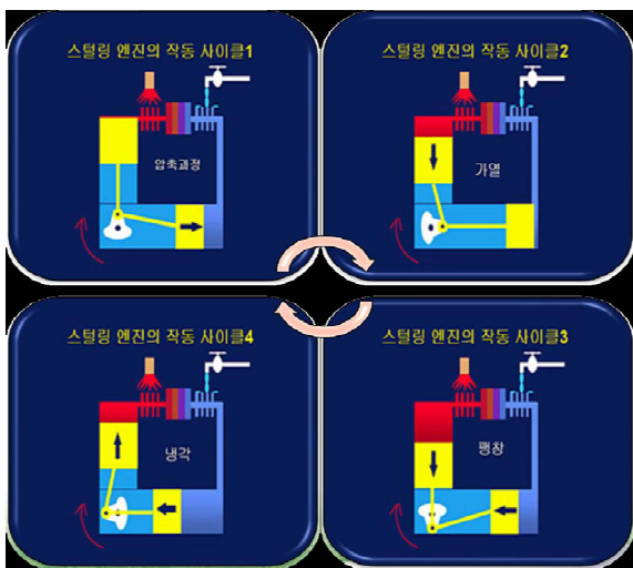
Fig. 2. Operation principle of stirling engine
