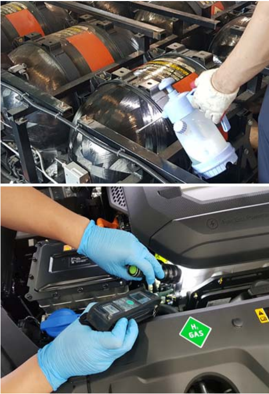
Fig. 4. Pressure vessels inspection of HFCEV.
