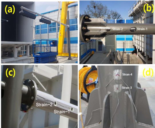
Fig. 5 Real wind tunnel test[(a)Attached Composite Material, (b)(c)(d) Attached Strain Gauge]
