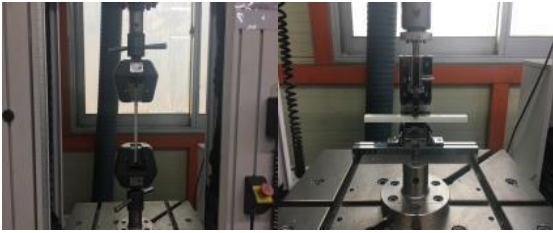
Fig. 3 Tensile and bending test
