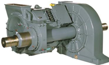
Fig. 2. 8200 electric locomotive traction motor.
