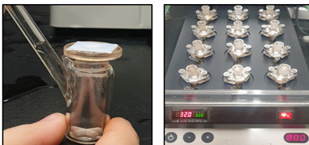
Figure 1. Franz diffusion cell with pig skin
