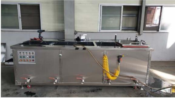
Fig. 1. Multiple ultrasonic cleaning equipment.
