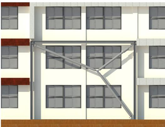
〈Fig. 5〉 Two-story toggle-brace-damper system
