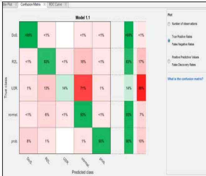
Fig 2. Confusion matrix contains true positive rates and false negative rates along with all classification of attacks
