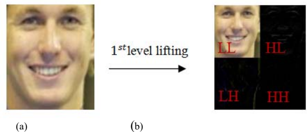
Fig. 3 (a) Original image, (b) 1-level 2-D lifting wavelet decomposition with an image from LFW dataset.
