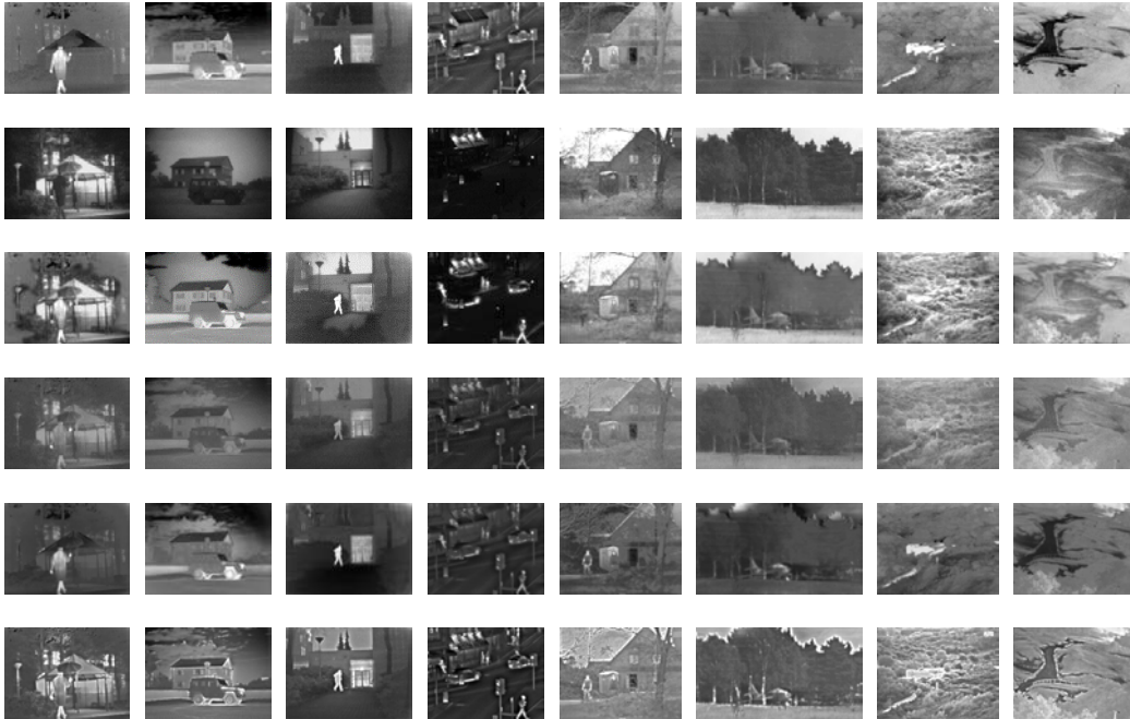
Fig. 9. Infrared and visible image fusion based on four typical methods. From top to bottom: infrared images, visible images, results of CNN, DLF, FusionGAN and Laplacian-GAN method.
